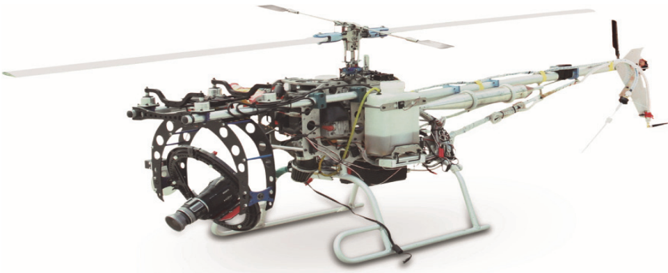
Fig. 2. SERVOHELI-40 small-size helicopter platform
